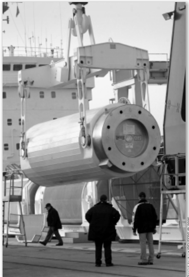
A container of vitrified nuclear waste being loaded on a cargo ship for shipment from Cherbourg, France, to Japan. Spent fuel from Japanese nuclear power plants is reprocessed in France and then returned to Japan.
